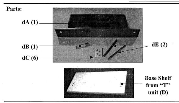
Arrange Drawer Catch (dB) and both Tracks (dE) on the inverted Base Shelf (D). Using Screws (dC), fasten Catch and Tracks to Base Shelf.
