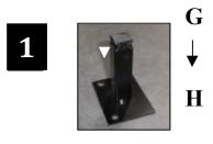
Assembling Legs: Insert caps (G) into leg [or casters] (H) bottoms.
